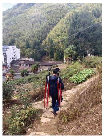
Figure 3: When carrying out 3D scanning, the machine needs the help of "targets" in order to map properly. Here a member of the AIM Team is carrying the targets to the proper place. Shot in Tongmu Village, Xingcun Town, Wuyishan City.
