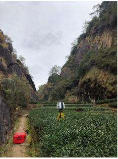
Figure 1: In order to achieve the best scanning result, the AIM Team uses a Leica long-range 3D terrestrial laser scanner to conduct 3D scanning in a tea plantation in Daoshuikeng, Mount Wuyi.
