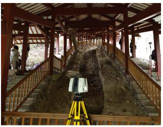
Figure 2: AIM Team uses a 3D scanner to map out the Yulinting kiln site of the Song period in Mt. Wuyi. Here the scanner is placed before the Dragon Kiln to scan from bottom to top. 圖二: AIM團隊利用三維掃描器在武夷山宋代遇林亭窰址進行三維掃描。 圖中掃描器立在龍窰的前端,由下而上進行掃描。
