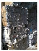
8. Shredded papers are not more than 8mm zigzag. The shredded papers are baled and then exported to recycled paper mills in South East Asia or China to manufacture recycled tissue.
